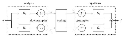
Figure 11: A subband coding system.
