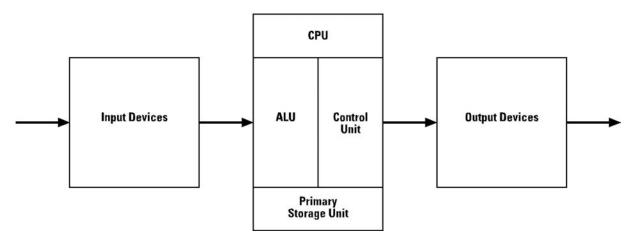
Figure 1: Building blocks of a computer.
