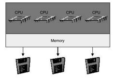
**Figure 7:** Symmetrical multiprocessing (SMP) architecture.
