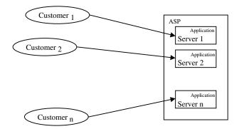
Figure 3: Application hosting deployment model.
