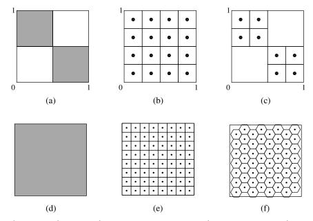
**Figure 6:** Advantages of vector quantization over scalar quantization (Gersho & Gray, 1991, Chapter 11): (a) the probability density function, (b) the scalar quantization for (a), (c) the vector quantization for (a), (d) the probability density function, (e) a square cell partitioning for (d), (f) a hexagonal cell partitioning for (d).
