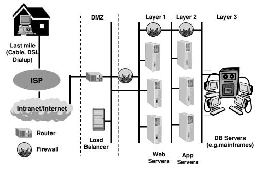
**Figure 4:** The Web infrastructure consists of many components, all of which must be considered for accurate capacity planning.
