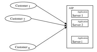
Figure 4: Application service provider deployment model.
