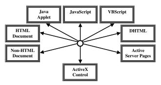
Figure 3: ActiveX integrates different Web technologies.
