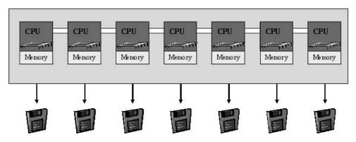
Figure 9: Massively parallel processing (MPP) architecture.
