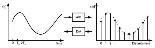
Figure 2: The relationship between a continuous-time signal and a discrete-time signal.
