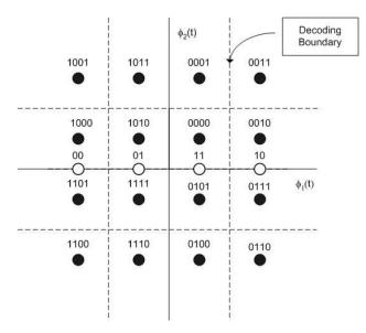
**Figure 4:** Signal space illustration of PAM and QAM signalling. The solid black circles are QAM and the white circles are PAM. The numbers above represent the mapping of bits to the constellation points.
