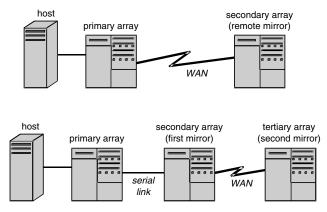
Figure 7: Remote mirroring configurations.
