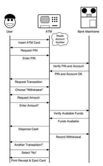
Figure 1: Sequence diagram for ATM withdrawal.
