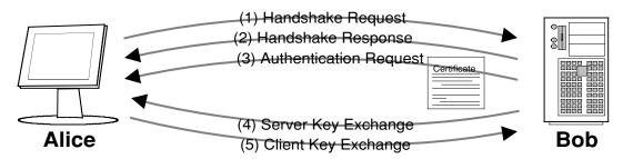
**Figure 2:** The SSL protocol. Alice (the client) and Bob (the server) exchange an initial handshake identifying the kind of authentication and configuration of the subsequent session security. As dictated by the authentication requirements identified in the handshake, Alice and Bob may exchange and authenticate certificates. The protocol completes by establishing a session-specific key used to secure (e.g., encrypt) later communication.
