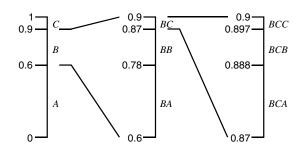
Figure 3: Illustration of arithmetic coding.
